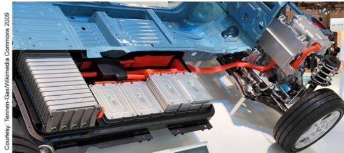
Figure 8: An early (2009) lithium-ion battery pack in a Nissan Leaf electric vehicle. At this time, the range was little better than 100 miles
