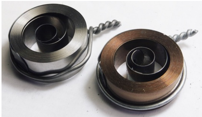
Figure 11: Two modern mainsprings, the preferential silver-coloured left-hand spring suggesting a higher yield steel hardened and tempered in an inert atmosphere
